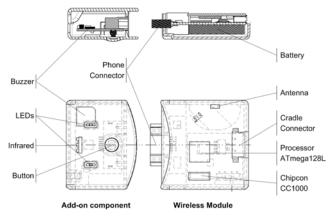
Fig 2: Buoy device schematics
