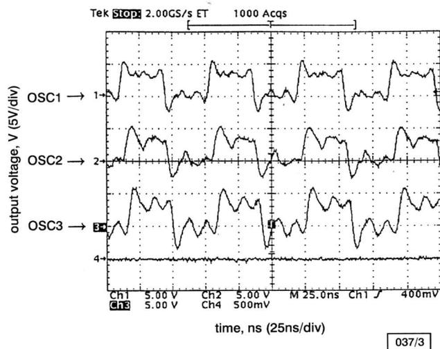
Fig. 3 Output waveforms from unidirectional loop of three IPLLs (with 31-stage EXOR-gate arrays)
